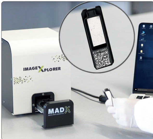
Fig. 1 Colorimetric spots on the biochip indicate the reaction of allergen and IgE antibodies. The signals' intensity is proportional to the amount of specific IgE antibodies bound to the allergen.
